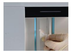
Running capillary blood through the sample probe directly is more convenient for the users in children's hospitals, etc. For Prediluted mode, UNICORN 5 has higher dilution ratio than other 5-part hematology analyzers, thus it brings a better mixing effect.
