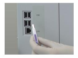
4 USB ports are located on the instrument's left side. They permit UNICORN 5 users to transmit data conveniently and connect with printers, keyboard, mouse, barcode scanner, etc.
