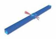
A most important technology is to ensure the WBC passing the laser beam one by one, when the sheath flow passes the unique designed square counting chamber. As the diameter of the WBC will not be too different from the diameter of the transversal surface of the chamber, the WBC are fixed in the middle of the sheath flow passing the square chamber constantly with a high speed. This Constant Linear Sheath Flow ensures the accuracy of the WBC counting.
