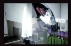
Each tube is picked up one by one from color-coded racks and gently mixed with built-in complete tube inversion mixing arm.
