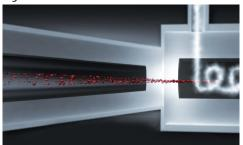
The DynaHelix Flow technology perfectly aligns WBC, RBC and PLT cells for high impedance counting precision using advanced hydrodynamic-focused sheath flow before passing through the aperture. In addition, the DynaHelix Flow totally prevent risk of coincidence or count of blood cell re-entry into the aperture using unique DynaHelix Flow stream. This newly-developed advanced DynaHelix Flow technology greatly improve counting precision and accuracy.
